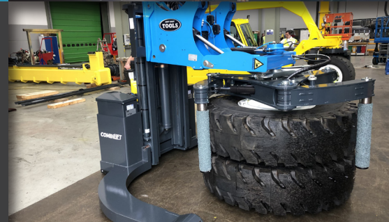
Precise 90° tilt, horizontal to vertical
