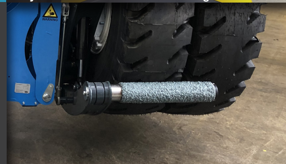
Stone-coated pipes ensure a safe grip
